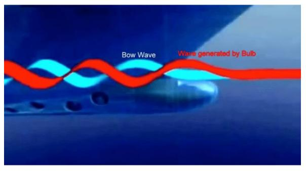
*Figure* **12.4.1** – *Concept of bow waves and bulb waves that cancel each other* [http://www.marineinsight.com/naval-architecture/why-do-ships-have-bulbous-bow/]
