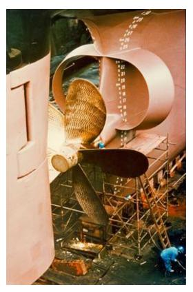
Figure 12.1.2 – Typical wake equalising duct [Scheneekluth]
