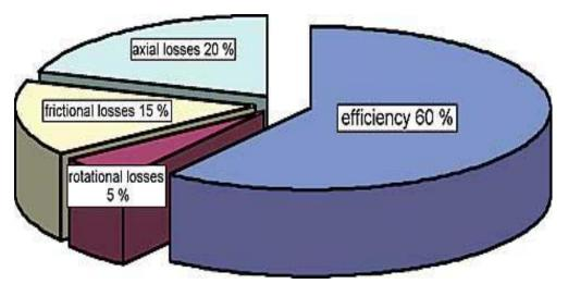
Figure 12.2 – Typical propeller efficiency and losses
