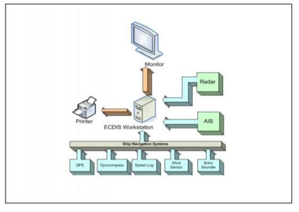
Figure 1.3: Concept of ECDS and its' integration with other system [Fredrik Larsson]
