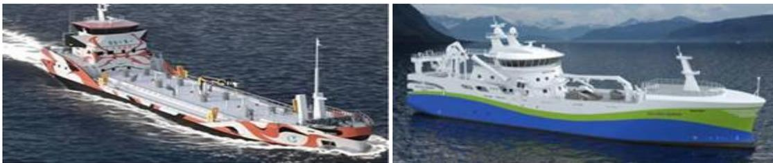
All electric ship - Zero-emissions tanker Corvus Energy propulsion system on board the all-electric Asahi Tankers vessel and on the right LNG-Powered Pursue Seine/Trawler
