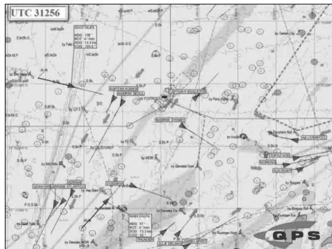
Figure 9 – AIS record of accident between Scot Isles and Waldi Halfa for e-learning platform Source: (Leonardo M'AIDER project, 2009-11)
