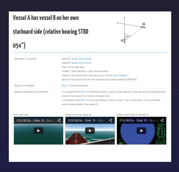
Different views are provided to support the training: bird's eye view, bridge view, radar screen view and also ECDIS view where necessary.
