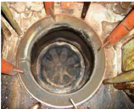
View of damaged cylinder liner with piston fitted.
