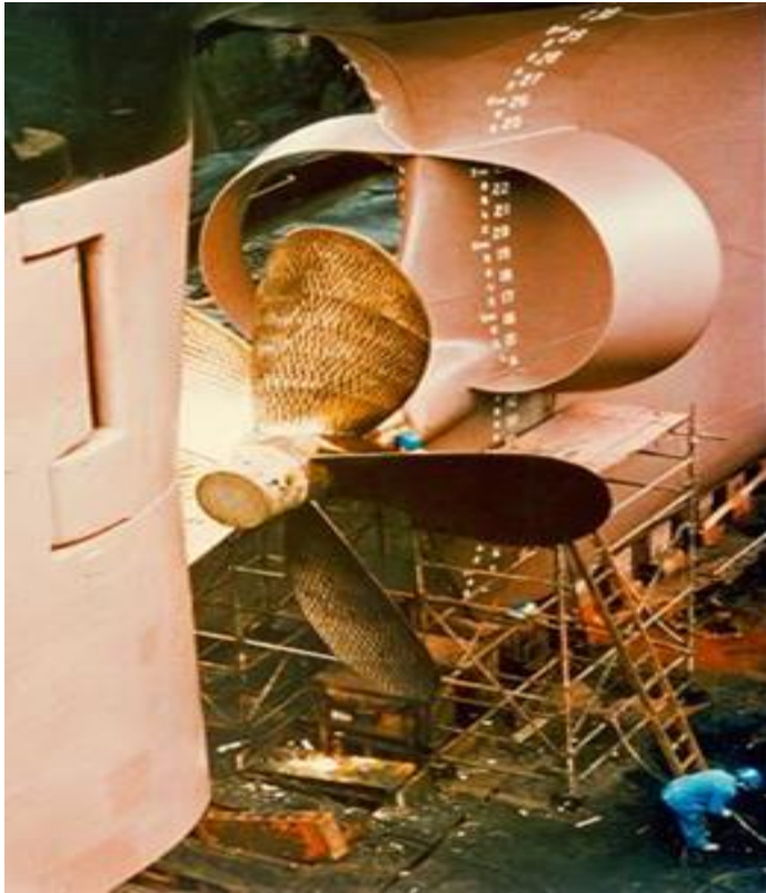
Figure 7.2: Typical wake equalising duct [Scheneekluth]
