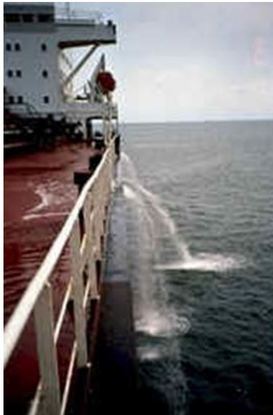
Figure 10.4: Ballast water exchange using flow-through method [Wikipedia]
